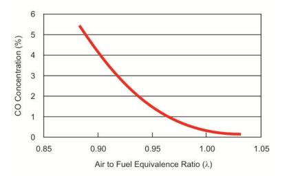
Figure 1. Sensitivity of LPG Emissions to A/F Ratio
