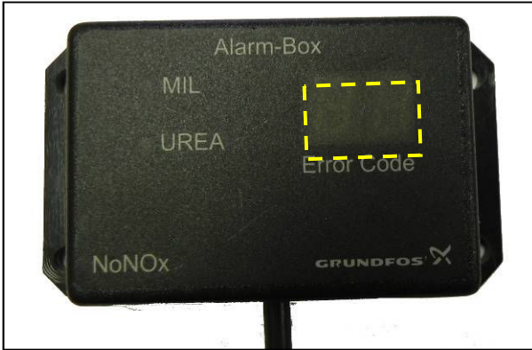
Figure 2: Urea Alarm Box Display
