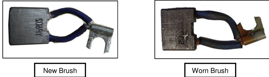
Figure 20: Comparison Between a New & Old Motor Brush
