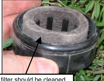
Figure 9: Dirty Air Filter
