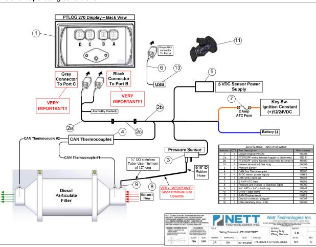
The PTLOG™270DPF is programmed to provide monitoring of DPF performance at all engine dynamic operating conditions. The display will provide information to the operator to schedule DPF cleaning ahead of critical failures to avoid unscheduled machine downtime. All warning and alarm messages are logged with date and time stamp.
