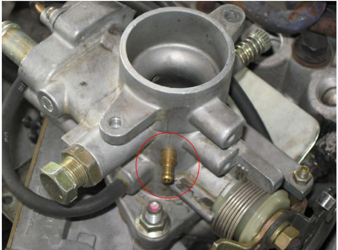
Figure 4b: Aisan Mixer – Location of vacuum port
