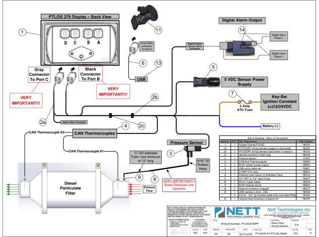
The PTLOG<sup>™</sup>270DPF is programmed to provide monitoring of DPF performance at all engine dynamic operating conditions. The display will provide information to the operator to schedule DPF cleaning ahead of critical failures to avoid unscheduled machine downtime. All warning and alarm messages are logged with date and time stamp.
