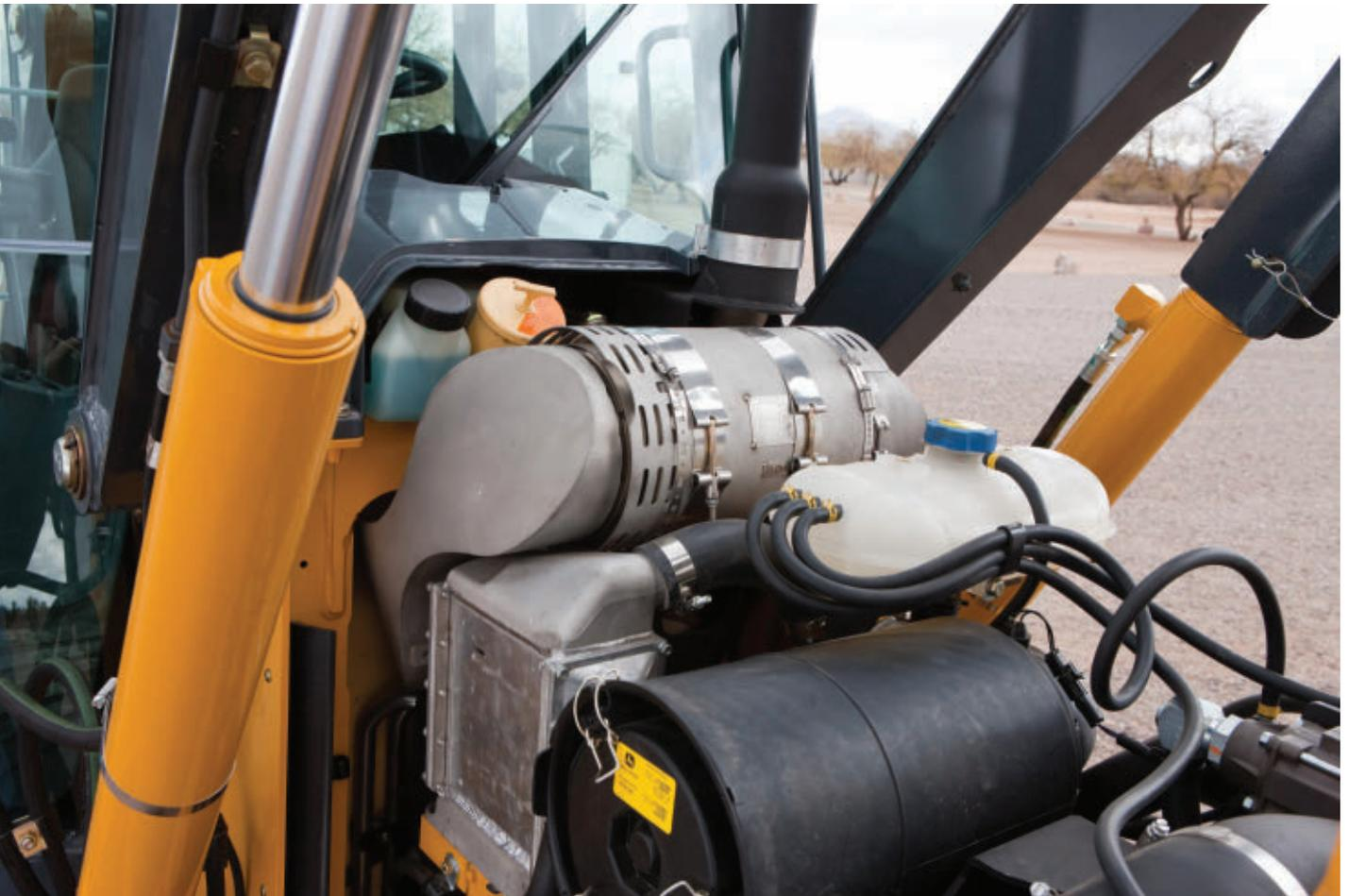
John Deere has announced a program to offer an actively regenerated diesel particulate filter for retrofitting “key legacy John Deere construction machines.” The program involves Nett Technologies VorTEQ 100 DPF. Nett has secured California Air Resource Board (CARB) Level 3 verification, which will carry the CARB 5 year/4200 hour mandatory warranty.
