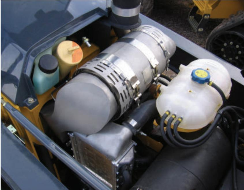
The Nett VORTEQ system utilizes a controller, monitor, and diesel burner to monitor filter condition and control regeneration. It is a stand-alone system and does not interact with the vehicle electronics or operator monitor systems.
