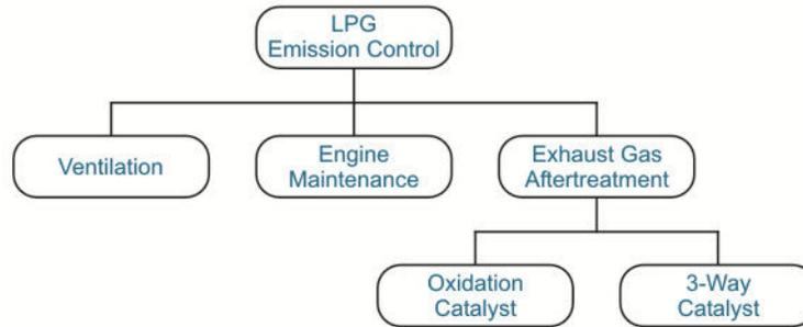
**Figure 2. Methods of LPG Emission Control**
